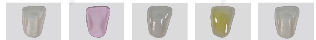
Original Zirconia Surface After Spray After Sintering Acid Etching After Acid Etching
